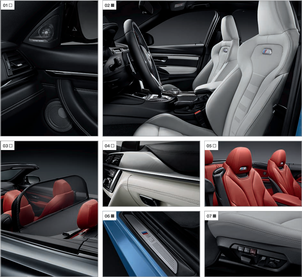
[ 01 ] Harman Kardon Surround Sound System with 600-watt digital amplifier, nine channels, vehicle-specific equalizer and 12 loudspeakers including centre speaker. [ 02 ] M seats 1 with bucket-style character 2 , integrated head-restraints, perfect body support from high side bolstering, backrest width adjustment and lumbar support. [ 03 ] The wind deflector effectively protects the driver and front passenger from draughts. When not required, it can be easily stowed behind the rear seats. [ 04 ] BMW Individual instrument panel finished in leather 3 (XTI): upper section in Black Walknappa leather and lower in fine-grain Merino leather in upholstery colour. Door panels trimmed in leather. [ 05 ] The neck-warmers provide the head and shoulders with pleasantly warm air for particularly comfortable driving when the roof is open. [ 06 ] The typical M doorsill finishers with model designation add to the sense of excitement about the driving experience as soon as you open the door. [ 07 ] Electric seat adjustment with memory function enables perfectly tailored seat positioning: seat height, backrest angle, fore-and-aft seat position and seat angle.
