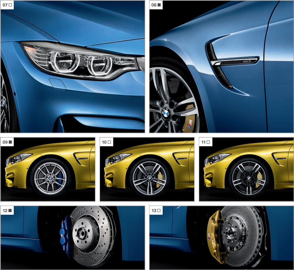
[ 07 ] Adaptive LED Headlights including low- and high-beam headlights, LED indicators and BMW Selective Beam (anti-dazzle High-Beam Assistant). [ 08 ] The striking M gills underscore the sporty look and, along with the integrated Air Breather, optimise aerodynamics. [ 09 ] 18" M light alloy wheels V-spoke 513 M with mixed tyres, forged. [ 10 ] 19" M light alloy wheels Double-spoke 437 M with mixed tyres, forged, burnished, Ferric Grey. [ 11 ] 19" M light alloy wheels Double-spoke 437 M with mixed tyres, forged, burnished, Black. [ 12 ] Through the use of various materials, M compound brakes achieve outstanding deceleration values and high stability as well as a long lifespan. [ 13 ] The M Carbon Ceramic Brake System offers even better braking performance and great stability. It also contributes to the further reduction of rotating mass.
